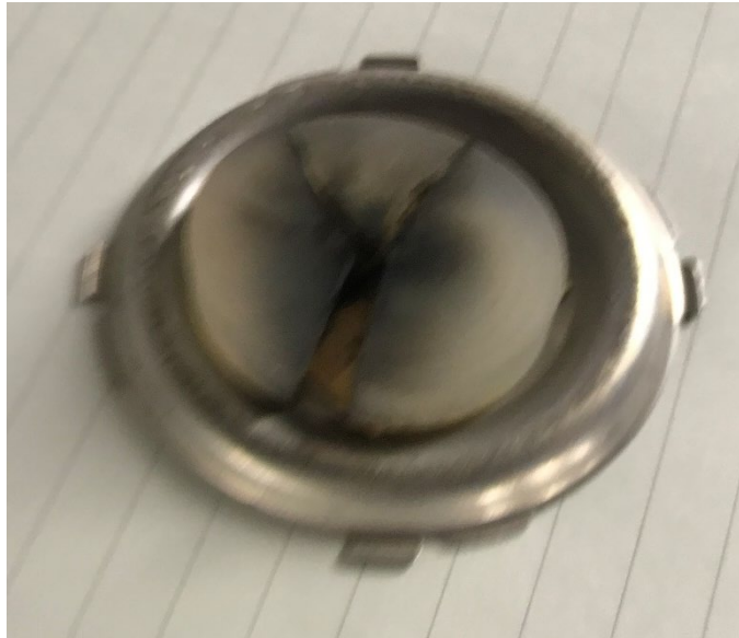
Figure 3 Damaged stand off/insulator on top of terminal control box
