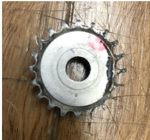
Figure 22 HE stripper sprocket spark damage
