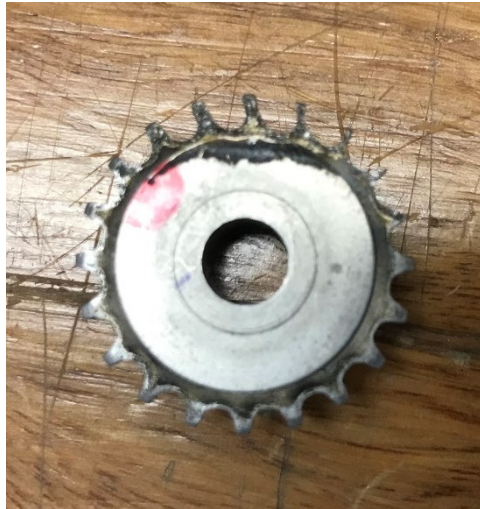
Figure 2 Damaged cog in mid-section stripper mechanism
