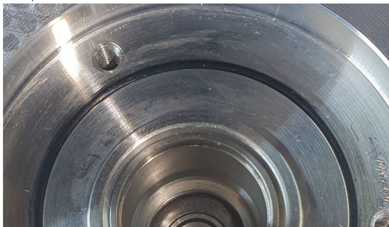
Figure 4 Dirt and debris on top bearing cover seal
