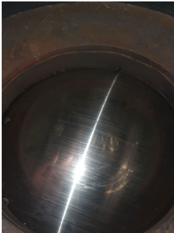
Figure 16 Scratches and scuffs on old ball valve
