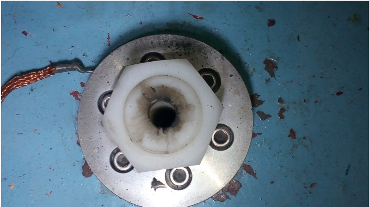
Figure 2 150kV beam focus nylon feed through (air side) showing blackened grease
