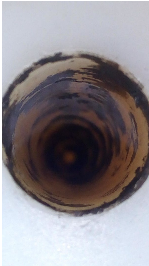
Figure 3 150kV beam focus nylon feed through HV cable (air side) showing blackened grease down bore
