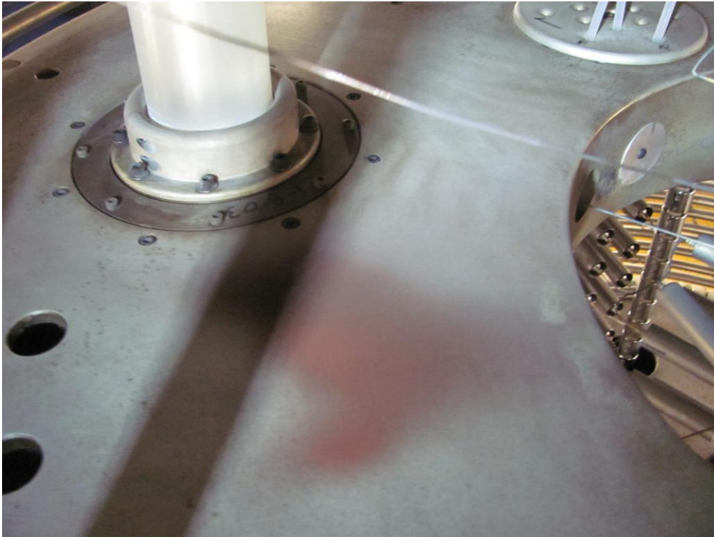
Figure 1 Residue under loose stringer
