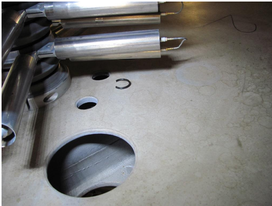
Figure 4 O-ring piece on casting U2
