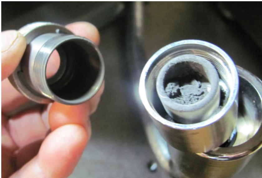
Figure 20 LE terminal ion pump connector
