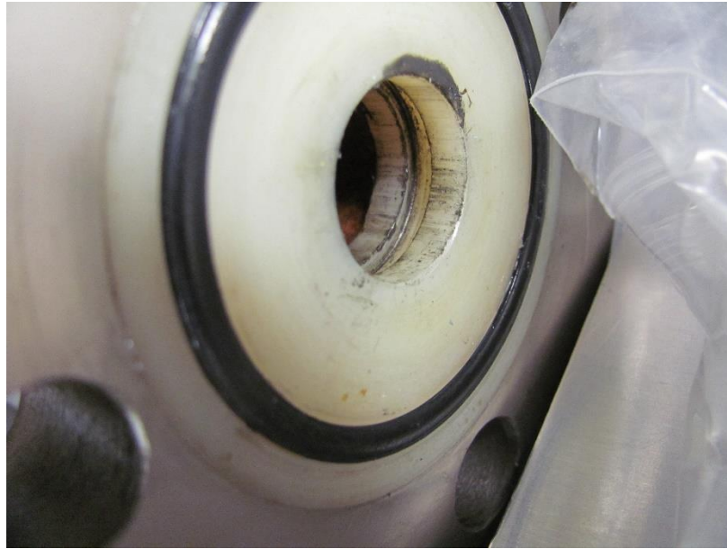
Figure 9 Location of missing o-ring
