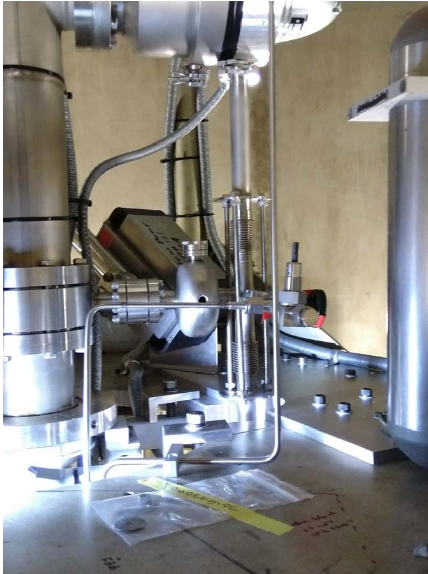
Figure 5 New gas stripper backing manifold with slot cut in terminal plate and extension piece to connect to the acceleration tube.
