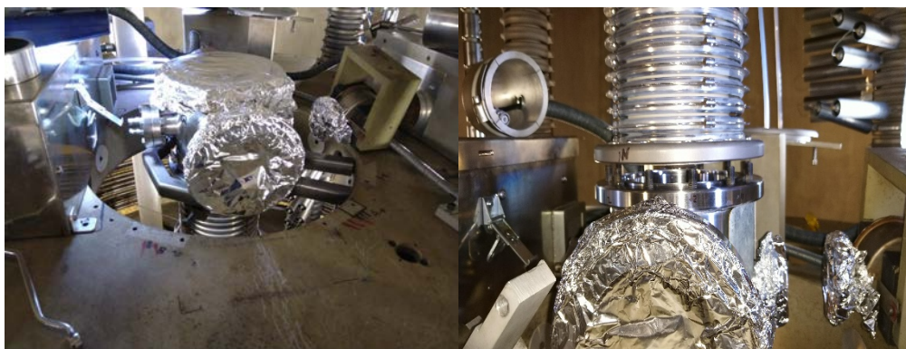
Figure 6 Installation of the new high energy stripper assembly
