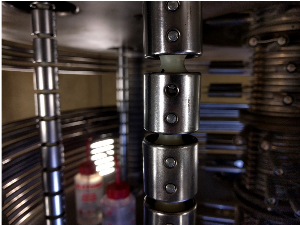
Figure 1 Loose rivet on chain 3
