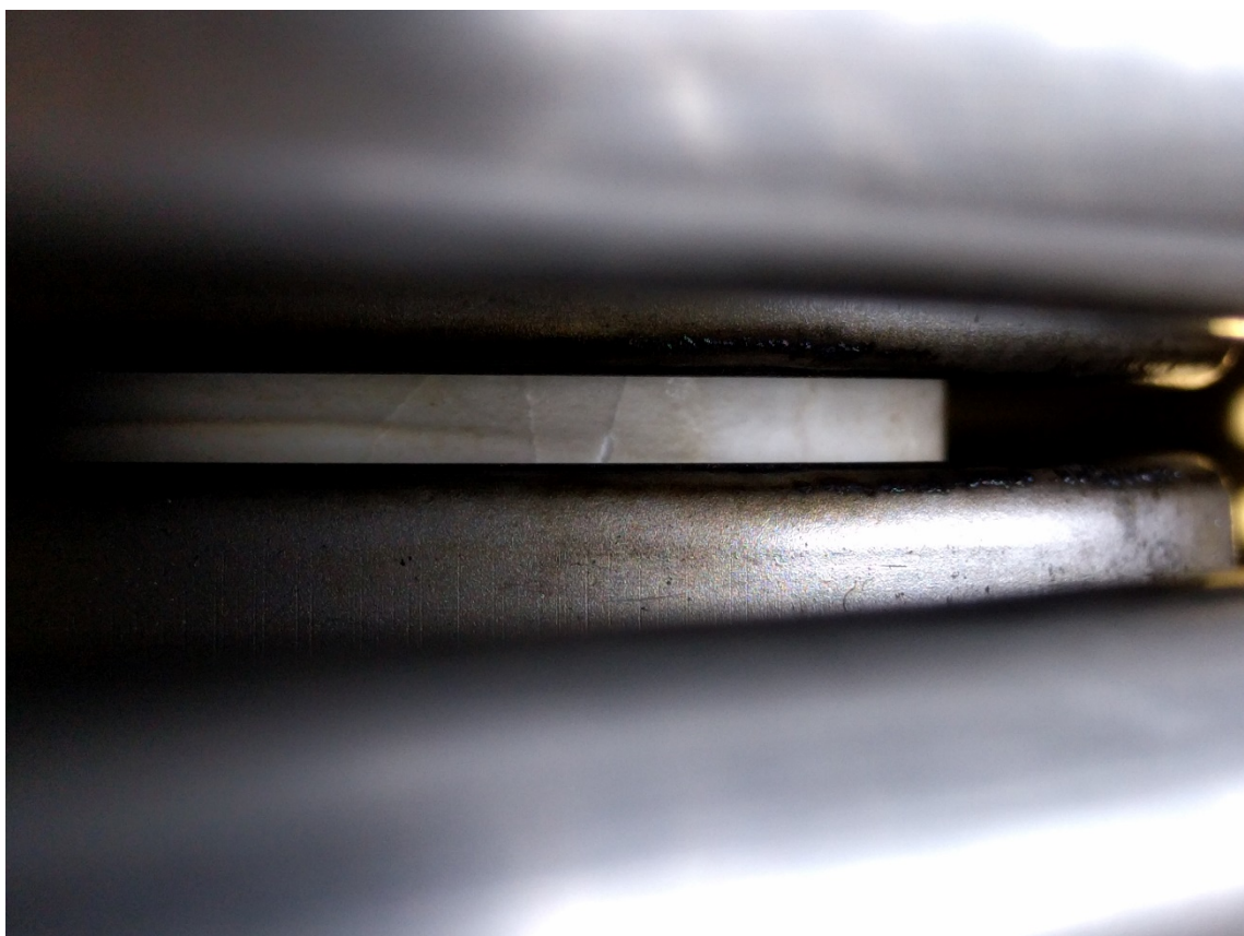
Figure 2 Unit 16 post B gap 1 cracks in ceramic
