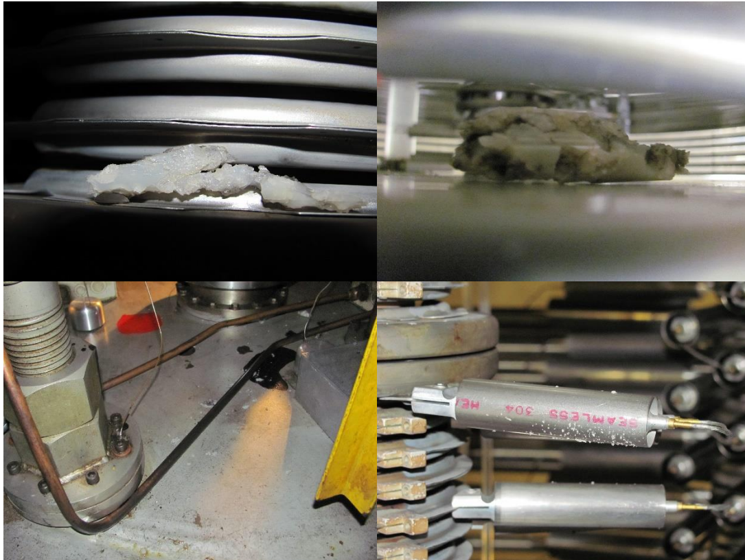
Figure 3-2 Debris field from shattered nylon shorting rod
