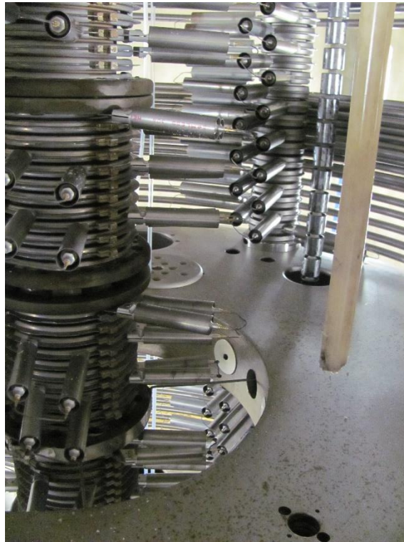
Figure 3-1 Shattered nylon shorting rod in unit 21
