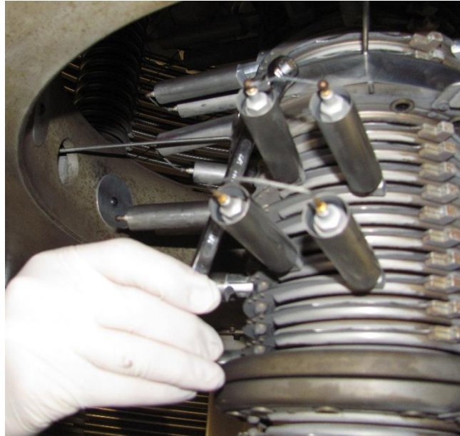
Figure 4-14 Loosening Spoke Clamp to Allow Rotation
