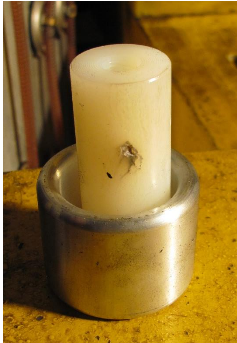
Figure 7-1 Supressor standoff spark damage
