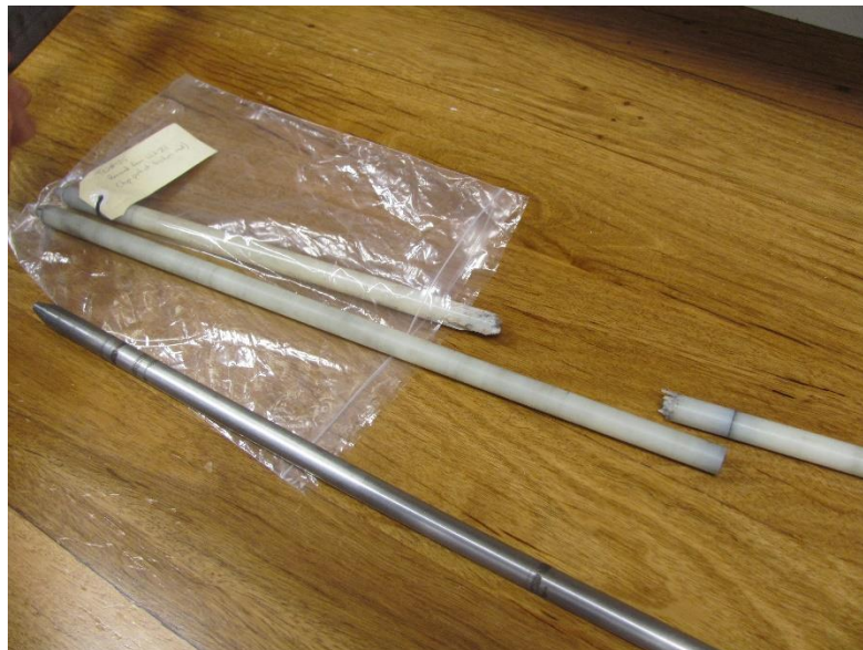
Figure 3-3 Comparison of shattered nylon shorting rod with good rod to show how much of the rod shattered. Also note the severe spark damage to the steel shorting rod at the spring contact points.
