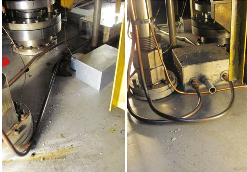
Figure 7 Nylon shards littering the bottom of the tank from exploded charging system standoff
