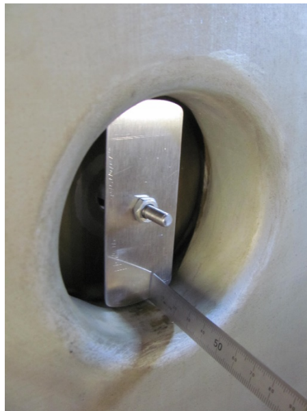
Figure 4 Modified spark gap behind mushroom-type CPO electrode
