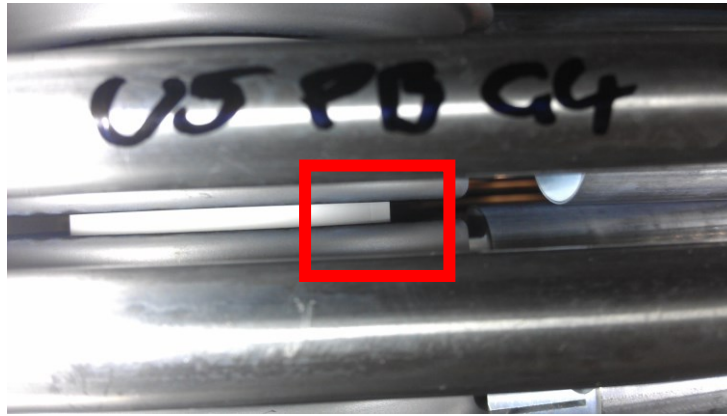
Figure 9 Ceramic damage unit 5, post B, gap 4
