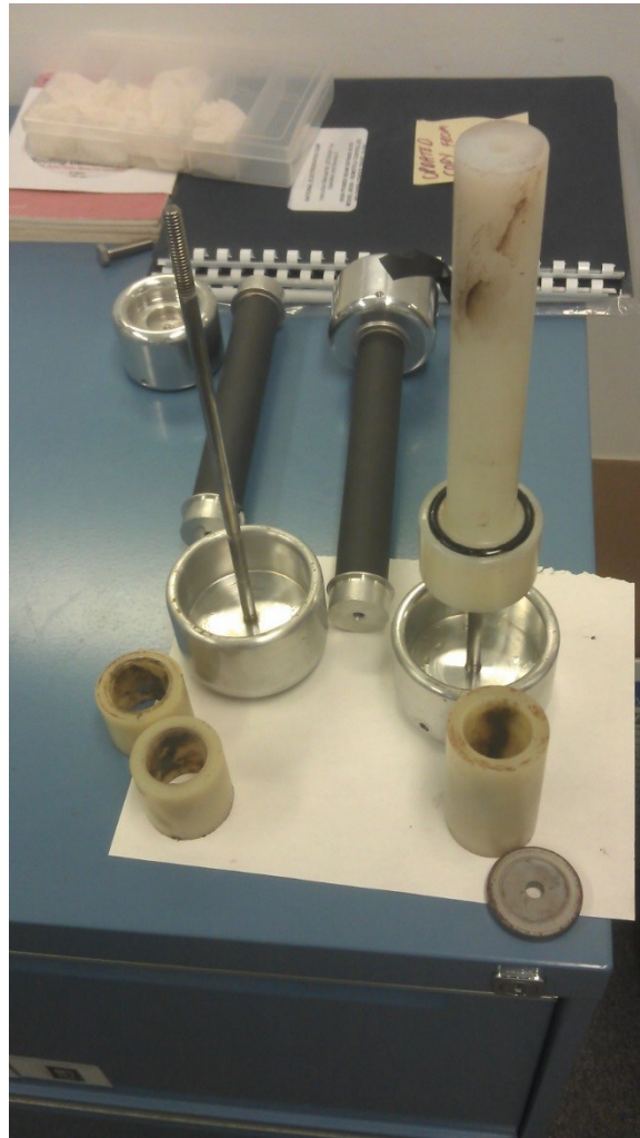
Figure 4 Damage on charging system feed thrus
