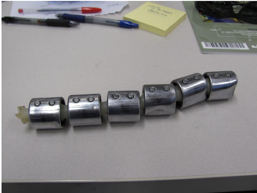
Figure 4 Six link piece showing link fracture
