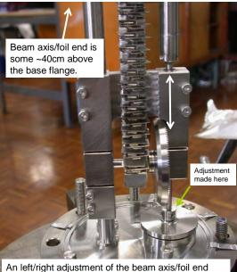
An left/right adjustment of the beam axis/foil end can impose compression or extension forces on the drive shafts and bearings, causing binding. The drive system thread and clamp feature requires adjustment to find the point of free rotation.
