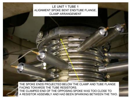
This allowed spark discharge to the resistor assemblies mounted across the first two gaps, although, possibly only during abnormal column or terminal voltage discharges.
