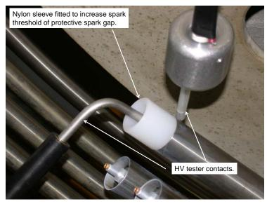
Where we were removing the tubes in Units 1 and 2, all the tube resistors would be removed and could be tested outside the machine at the workbench. The original resistor specified tolerance of our resistors is 2%. We had a maximum deviation from the specified value of +3.2% and -11.3% for the tube resistors of which the worst five were replaced and for the column resistors a deviation of +8.55% and -1.52% of which two were replaced.
