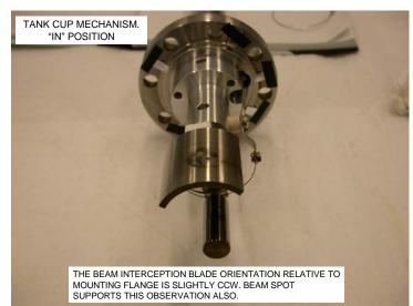
Weisser and others examined the beam spots on the cup and it was decided that the position of the cup element could also be better centred across the beam axis. This was achieved by fitting a new spacer 0.060" longer than the existing one.
