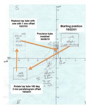
Post opening tests show the new precision tubes have significantly changed the position of the beam entering the accelerator to be much closer to the geometric
