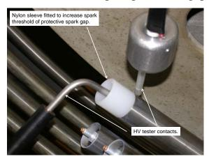
and the current noted. The testing of individual column post resistors in Unit#1 was undertaken. There was up to 6% variation in the current values. The original resistor specification was 2%. Time did not permit more extensive testing. We plan to do more and hope to better understand these initial observations.
