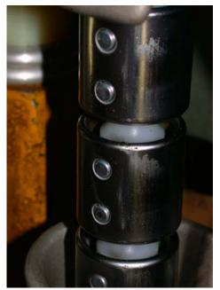
Heartened by the success the crew decided to run the chain for a few more hours, whenever there was a break in the work program, usually overnight. Chain #1 ran a total of 96 hours of which the initial 14 hours were with oiling. There were no signs of white powder and the charging test found that voltage and current were normal.
