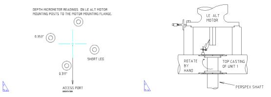
The coupling was installed to the motor shaft and then the micrometer was used to reposition the motor and the aluminium stand bolts were tightened. The coupling flange was then bolted to the casting alternator flange.
